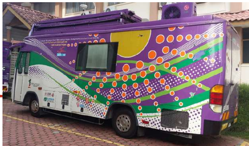
CETREE Green Bus (Vegetable Oil Based Genset – 8 Kwh)
